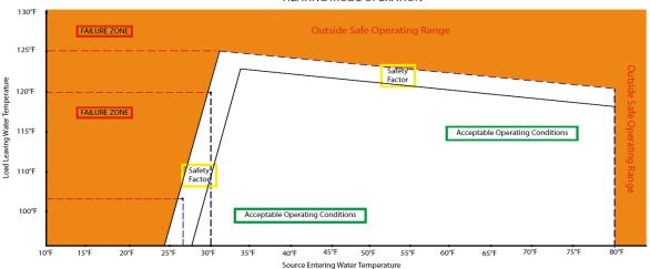
SCROLL COMPRESSOR OPERATING CONDITIONS (WATER TO WATER) HEATING MODE OPERATION
